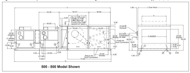
Figure 43.2 - DCS Separated Combustion Cooling Package Unit Dimensions with Blower Type I, J, or K
