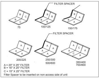
Figure 47.2 - Filter Replacement Arrangement for Blower Size (Digit 16) I, J, K, and L
