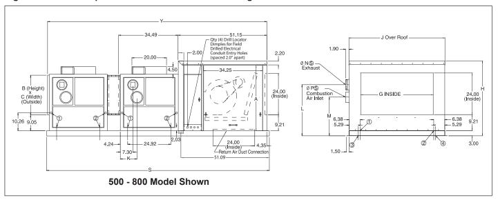
Figure 42.2 - DCS Separated Combustion Cooling Package Unit Dimensions
