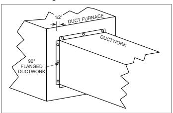
Figure 5.3 - Recommended Field Installed Discharge Duct Configurations for Blower Package Units
