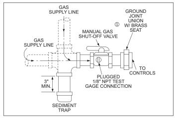
① Manual shut-off valve is in the "OFF" position when handle is perpendicular to pipe.
