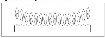
Figure 50.2 - Floating Flame Condition
