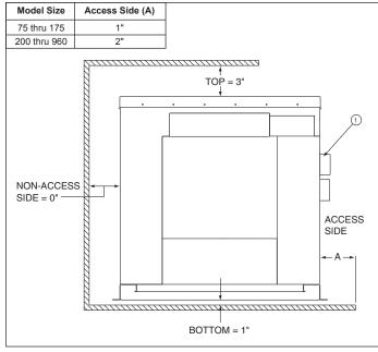
① A 3" minimum clearance to combustible material is required from the vent collar.
