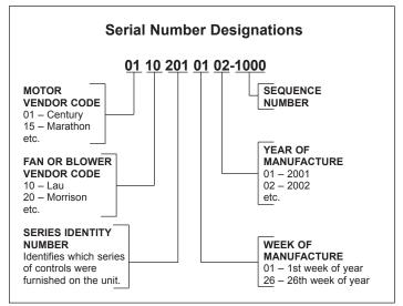
① Serial number format subject to change. When contacting the factory for replacement parts, always have the actual serial number ready from the unit(s).
