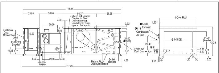
Table 43.1 - Indoor Separated Combustion Unit Dimensions with Blower I, J, K, or L (All dimensions in inches)
