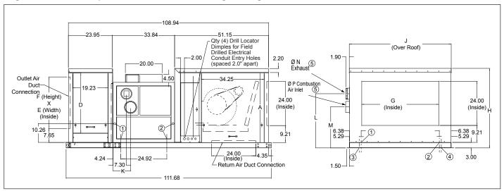
Table 42.1 - Indoor Separated Combustion Unit Dimensions (All dimensions in inches)
