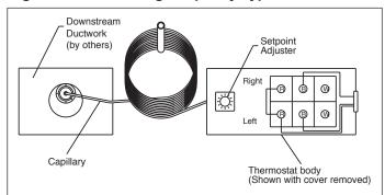
b) Two-stage Electronic Type Thermostat - Includes a field installed discharge air sensor. The thermostat body is field installed remotely and includes the discharge air set point adjuster that must be field set. Refer to Literature 5-577 latest revision.
