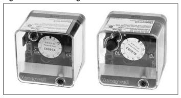
the gas controls have been damaged by the high gas pressure and then reset the switch to allow the unit to operate when gas conditions are returned to the allowable range of the pressure switch. The pressure switch range is 2" to 16" W.C. and should be set to insure that the maximum manifold gas pressure is not exceeded (3.5" W.C. for natural gas, 10" W.C. for propane gas).
