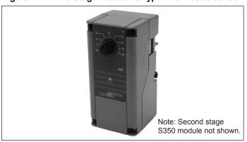
c) Electronic Modulating Discharge Air Thermostat – Includes a field installed mixing tube and discharge air sensor field installed in duct work. The set point adjuster is field installed remotely and must be field set. Refer to Literature 5-578 latest revision.
