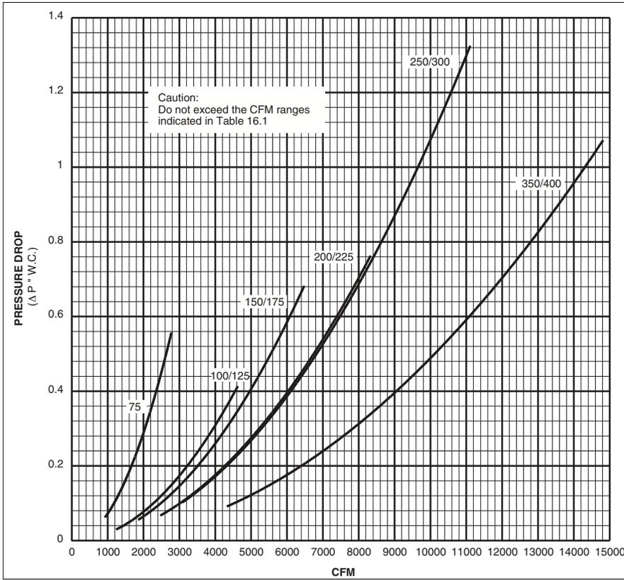
Figure 17.2 - Indoor Duct Furnace With Baffle Pressure Drop vs CFM curves
