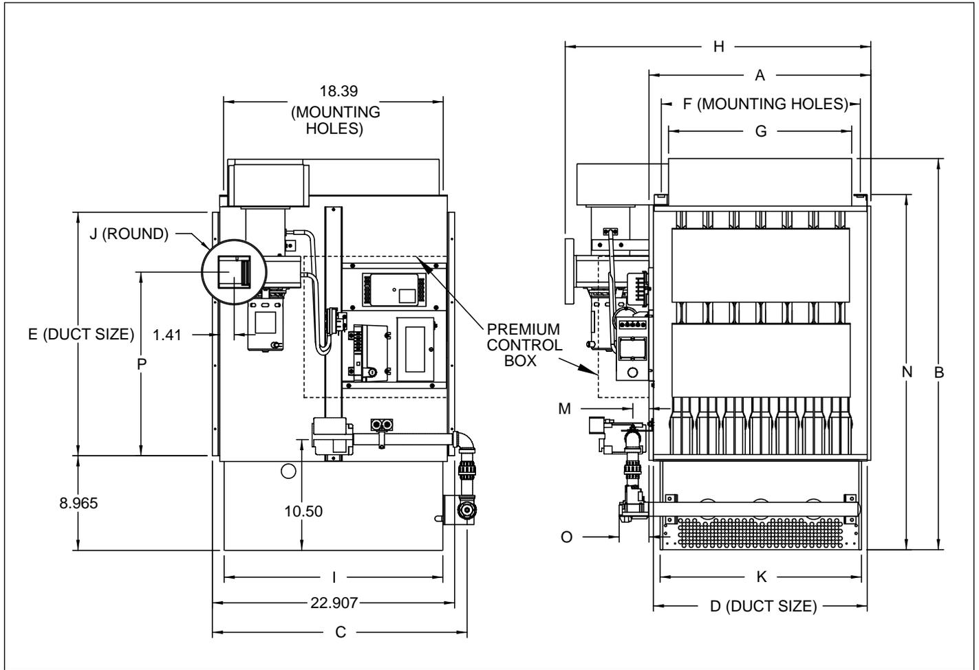
Table 15.1 - Indoor Power Vented Duct Furnace Dimensions
