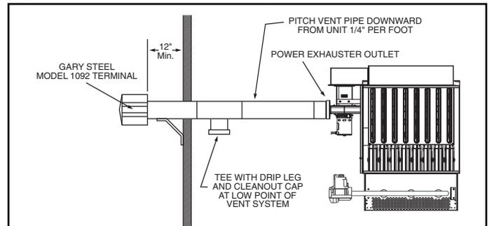
**Figure 7.3 - Venting Through Combustible Walls**
