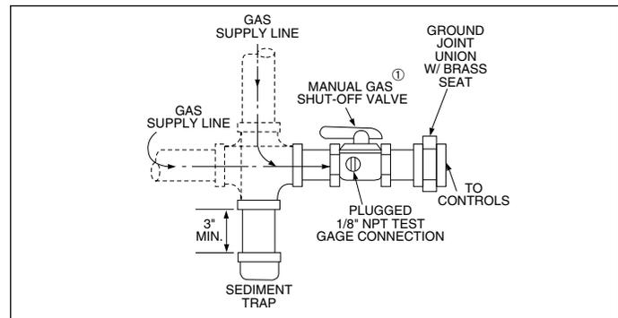
Ⓜ Manual shut-off valve is in the "OFF" position when handle is perpendicular to pipe.
